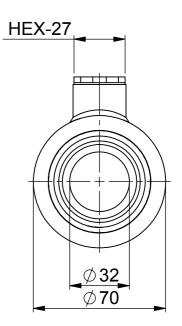
Top view of the stem without the plug
