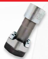
The HAELOK® fitting, type "FS" (SAE flange), is used for a straight connection with a counter flange. SAE Flanges according to DIN ISO 6162-1 (Code 61) pressure class 3000 PSI / 207 bar. The flanges are supplied with O-ring and two half flanges. Half flanges can only be connected to each other with a connecting plate. The advantage of this connection is the freely rotating assembly.
