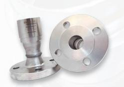
The HAELOK® fitting, type "FD" (Flange DIN), is a detachable connection to valves, pumps and tanks. We offer from stock PN40 flange connections according to DIN 2633, standard sizes range from DN 20 to DN 50. The flanges are supplied without gaskets and fasteners. The hole pattern also fits flanges of the PN16 and PN25 series.
