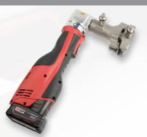
The press tool consists of a hard anodised housing and a maintenance-free closing mechanism. The battery-powered hydraulic unit is state-of-the-art and guarantees a perfect and carefree installation in any situation. By simply turning the horns, the press tool can cover the range from 6 mm to 13.5 mm. All HAELOK® press tools are tested and CE-conform.
