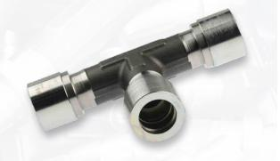
The HAELOK® fitting, type "T3" (Equal-T), is used as a connection between three pipes. The fitting consists of a total of four permanently mounted components; a base body and three press rings. Special designs with unequal outlets (TR/T-reduced) are possible within limits.
