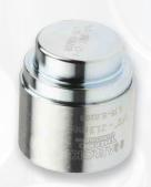
The HAELOK® THERMO fitting, type "EC" (End Cap), is used as a district heating pipe closure. It is especially optimized for high pull-out forces, temperature changes and for use according to the current specifications of AGFW FW 449 The fitting consists of two fixed components; a base body and a press ring.
