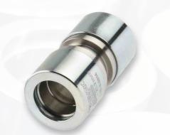
The HAELOK® THERMO fitting, type "SR" (Straight Repair) is used for a straight connection of two district heating pipes. The fitting can be moved over the whole pipe to carry out repairs. It is especially optimized for high pull-out forces, temperature load changes and for the use according to the current specifications of AGFW FW 449. The fitting consists of three fixed mounted components; a base body and two press rings.
