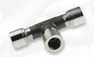
The HAELOK® fitting, type "T3" (Equal-T), is used as a connection between three tubes. The fitting consists of a total of four fully assembled components; a base body and three press rings. Special designs with unequal outlets (TR/T-reduced) are possible.
