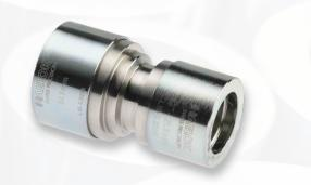
The HAELOK® THERMO fitting, type "RE" (Reducer) is used for a straight connection of two district heating pipes with different diameters. It is specially optimized for high pull-out forces, temperature changes and for use according to the current specifications of AGFW FW 449. The fitting consists of three fixed components; a base body and two press rings of different sizes.
