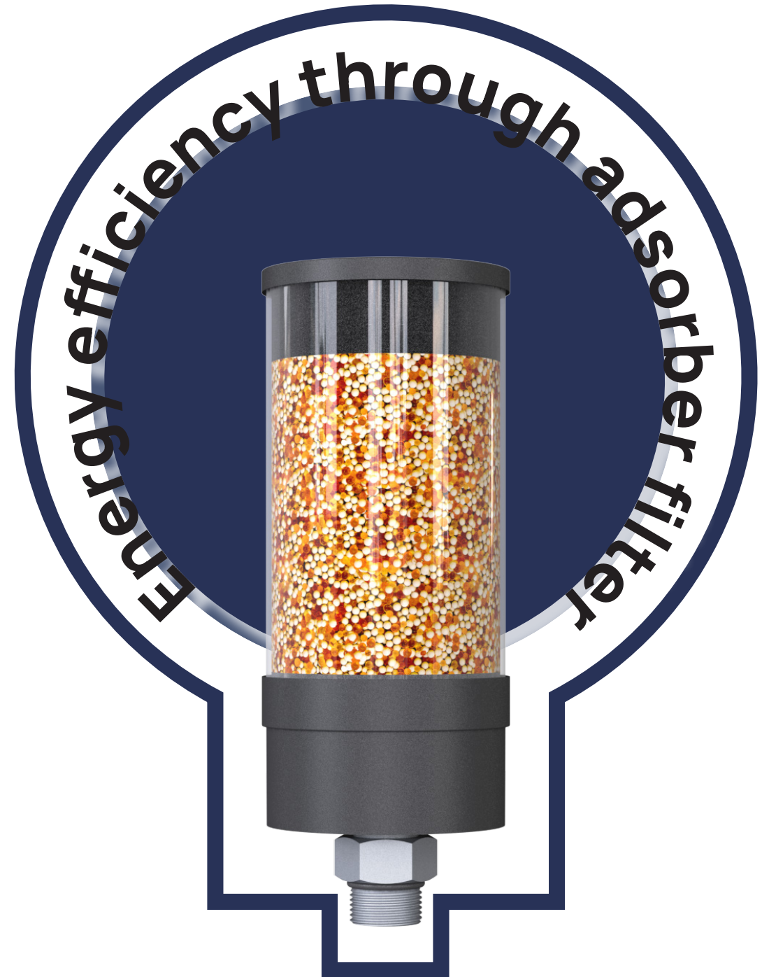
2. Hydraulic oil is removed from the tank, the oil level drops and the pressure is equalized by incoming air. The adsorber separates moisture up to 2% RH (on average 10% RH).
