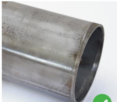
Good pipe ground
