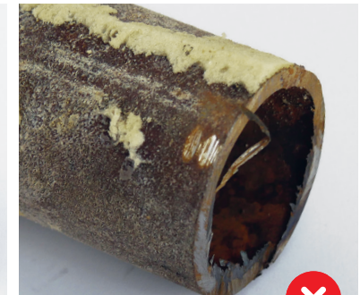
Plastic casing pipe not deburred, residues, surface cannot be assessed
